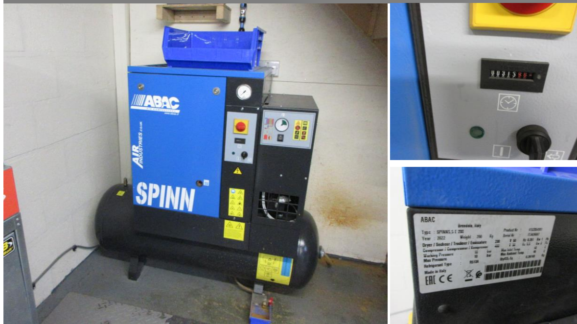
ABAC receiver mounted packaged air compressor, type SPINN5.5E 200, serial no: ITJ626067, run hours 315 (2022)
