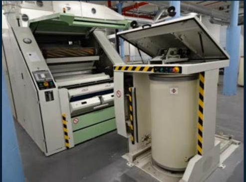
Aramid fibre fine counts spinning unit: 2 off LMW Lakshmi LC361 1100mm Cards (2016) 1 off Zinser 670 Flyer Rover 108sp (2001) 1 off Lakshmi LRJ9/SX 1200sp Spinning Frame (2016)
