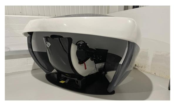
Full motion simulation, Variable driving position, 200 degree wrap around screen, Thrust, Pitch, Roll & Heave capabilities
