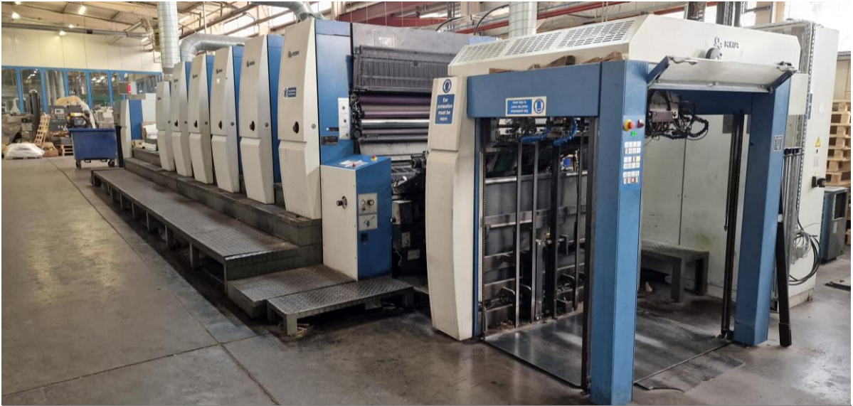
KBA Rapida 105- 5+L 5 Colour B1 sheet fed printing press (2008)
