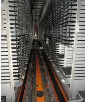
ACMF phial tray withdrawal system (1of2)
