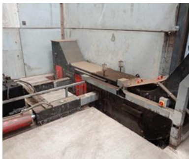
Hydraulic dual ram driven walking floor
