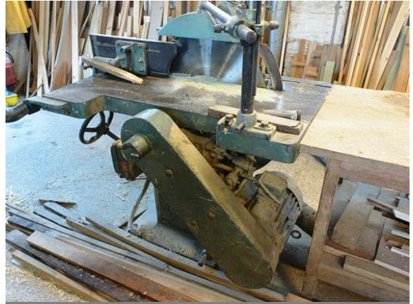
A Cooksley table saw, blade dia 24", 3 phase
