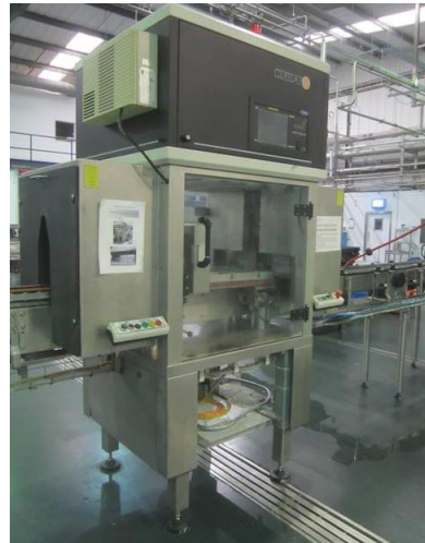
Heuft Spectrum TX stainless steel bottle squeezer X Ray detection machine, X Ray detectors
