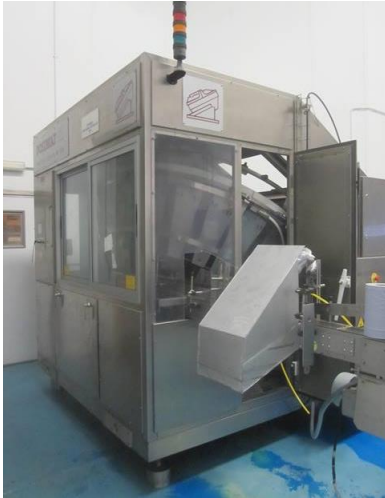
Posimat stainless steel automatic plastic bottle unscreamer / dispenser, model N20, (2008)
