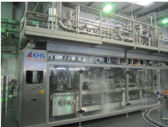
KSH stainless steel Asbofill aseptic 24 nozzle bottle filler, with max fill capacity per bottle of 125ml to 750ml, type 610/03, serial no: 610/03-12N016 (2007)
