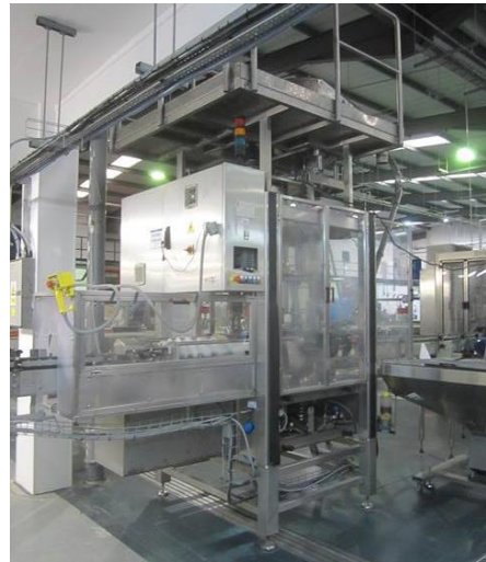
Andre Zalkin stainless steel 6 head 38mm rotar capping machine, type CA.6.360.NG, serial no: 24431 (2008)
