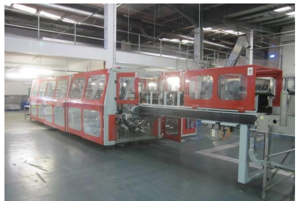
Ocme N40 cardboard packer, type Altair N40, serial no: 0800039A02, 4 lane adjustable width infeed conveyor, cardboard dispenser, packing station, Nordson glue station
