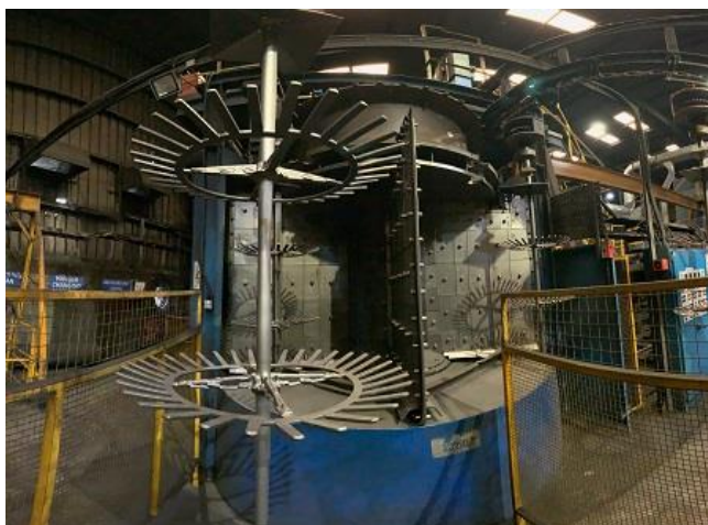
Spencer & Halstead rotary 4 compartment shot blast machine
