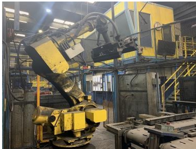
Fanuc R-200ib multi axis loading insert robots
