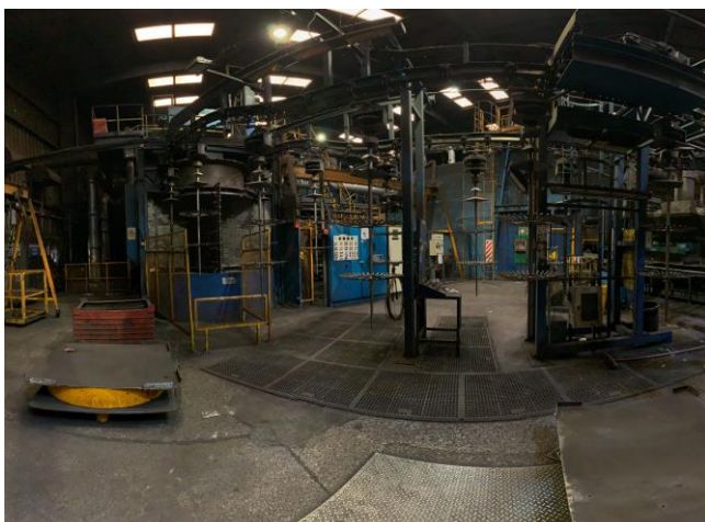
Spencer and Halstead rotary shot blast machine with monorail infeed and outfeed system
