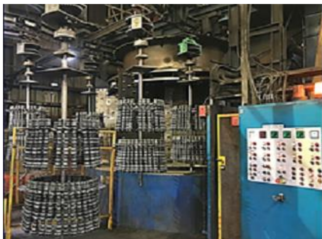
Spencer & Halstead rotary 4 compartment shot blast machine
