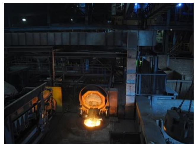
Inductotherm Powertrack Induction Furnaces, 4 tonne capacity 2,500 to 3,000Kw, 3-off (1991-2018)
