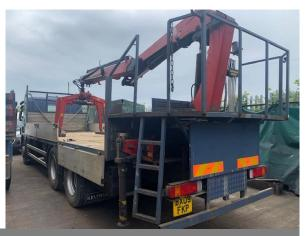
Scania P-SRS D-Class, 8,867cc Diesel flatbed brick/block lorry, registration number: BX09 FKP, 3 axle rigid, Test valid until 30/04/20, Mileage: advised circa 250,000kms ,with HMF 1420K1 rear mounted block crane, S/N: 1050087 LOLER Certified, date of test 25/06/19
