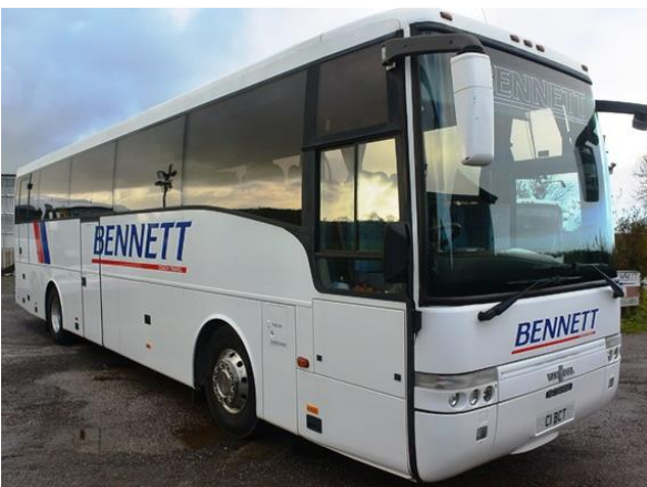
Scania K114 Van Hool Alizee II 49 + 4 executive seater Euro 4 coach, reg no C1 BCT (2003), MOT 6/12/20, tachograph reading 748,307 kms, fitted central toilet, air con, 7 speed comfort shift, with seating and floor plan to configure into 53 seater
