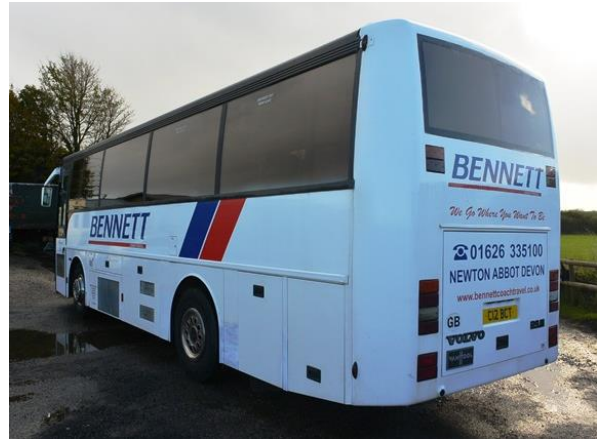
Volvo B9M Van Hool 38 executive seater Euro 4 coach, reg no C12 BCT (1996), MOT 30/9/21, tachograph reading 781,610 kms, fitted rear toilet, air con, TV, 6 speed box
