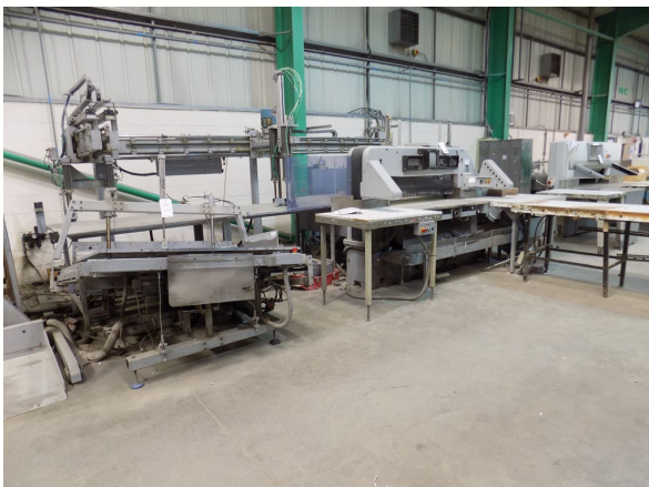
Schneider paper guillotine with pick & place, jogger & stacker
