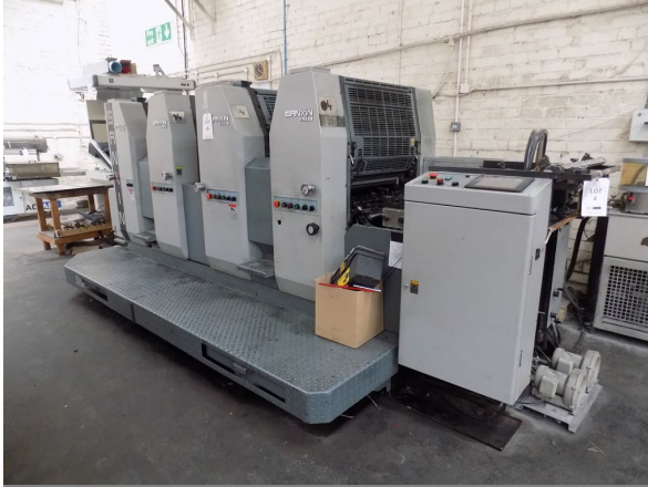
Saxin four colour sheet fed off-set printing press
