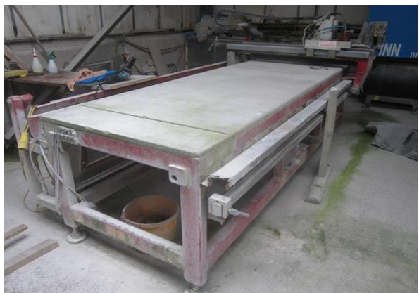
Ghines Systar bench type stone router s/n: Sys 0007 (2006) 3phase, (currently out of commission)
