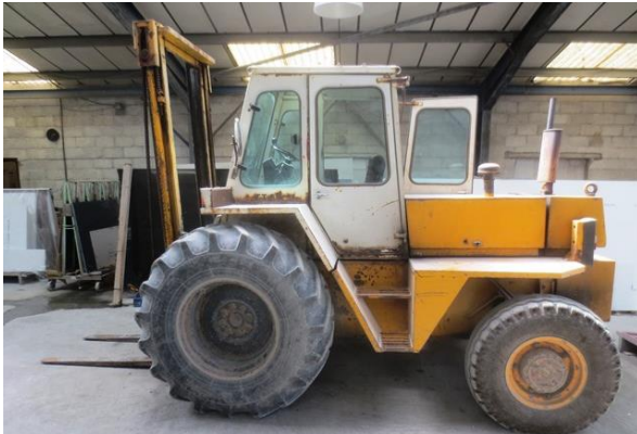
Coventry Climax diesel powered tough terrain, all terrain Dual mast FLT
