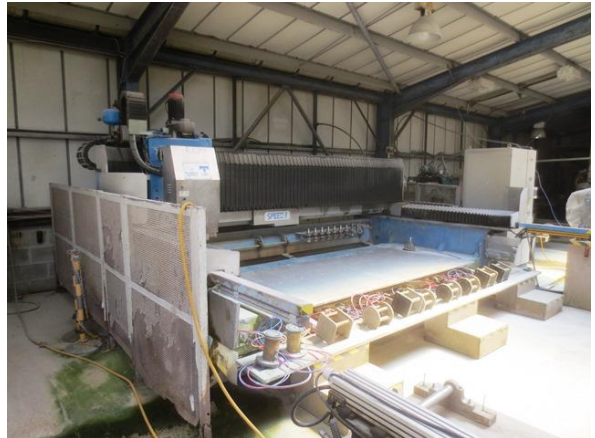
CMS Tension Nominal 400, Brembana Speed 3, bridge type CNC machine centre s/n: 2771 (3phase), with GF Fanuc Series 180i-M control and Viale 5210 coding unit and 12 tool holder capacity (2001)
