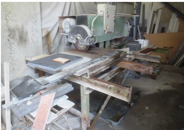
Twin blade, steel-frame mounted stone saw, approx. distance between blades 1.2m, 3phase (constructed on-site)
