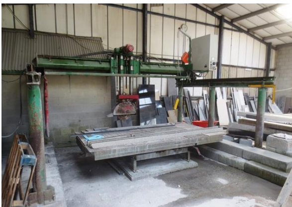
Spiel Vogel 356 S, floor bridge type saw, mounted s/n: 90NR4142, Approx. floor plan 3x4m
