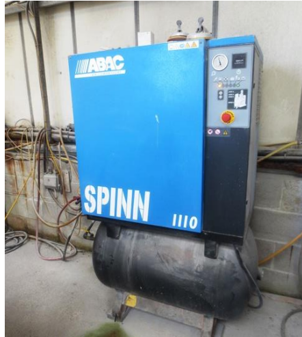
ABAC Spinn 1110 receiver mounted air compressor s/n: 324809 0004 (9534 hrs) (3phase)
