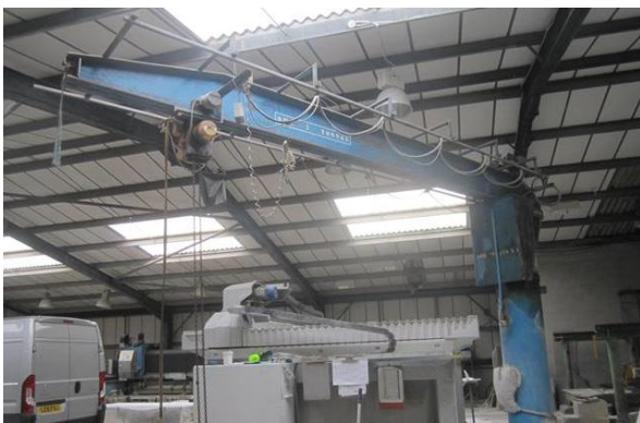
Floor-mounted pillar job crane
