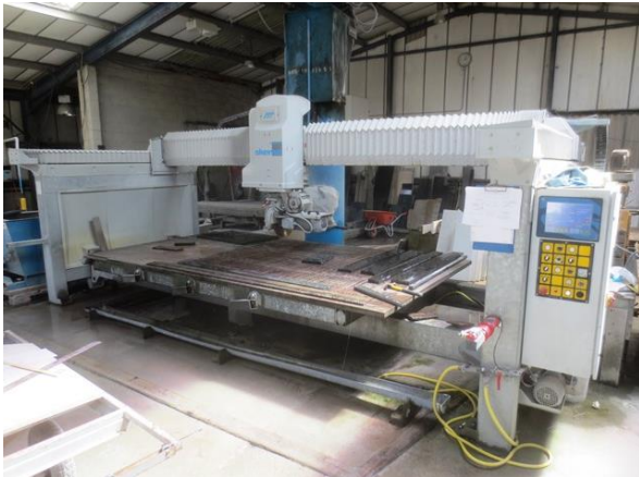
Denver, 3 axis Skema bridge type saw s/n: 4210513 (2013), (2600kg) with Syel V10 control
