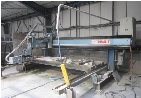
Thibaut T50 bridge type works centre s/n: 4 (1993), 3phase
