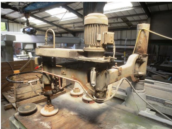
Unbadged radial arm face polisher (3phase), electrical lift, manual articulated arm
