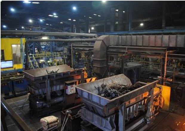
Vibratory Hopper Feeders 2-off with outfeed to furnaces
