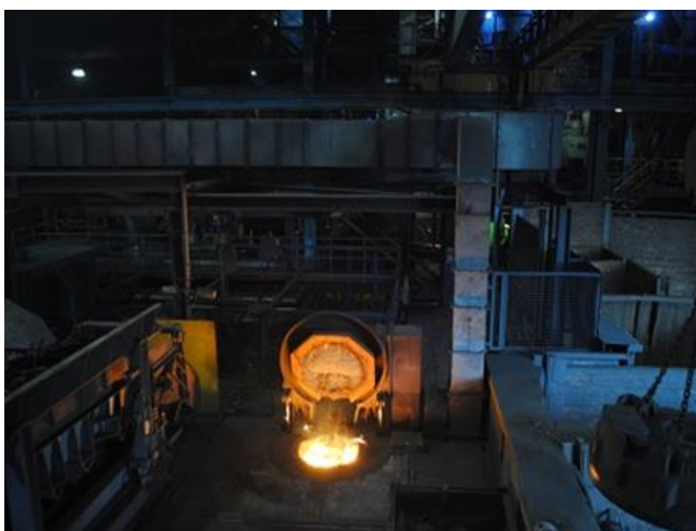
Inductotherm Powertrack Induction Furnaces, 4 tonne capacity 2,500 to 3,000Kw, 3-off (1991-2018)
