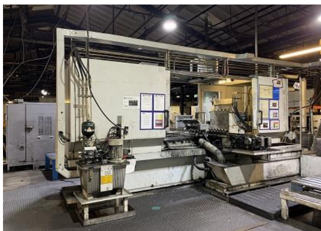
Tibo multi spindle gun drills, 6-off 2001 – 2012
