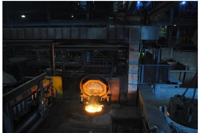
Inductotherm Powertrack Induction Furnaces, 4 tonne capacity 2,500 to 3,000Kw, 3-off (1991-2018)
