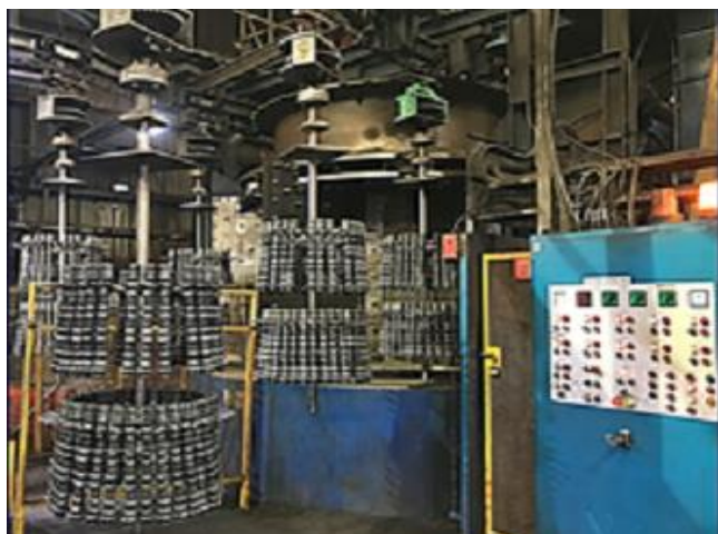
Spencer & Halstead rotary 4 compartment shot blast machine
