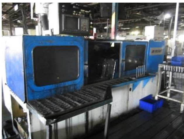
Mollart multi spindle gun drills, 3-off (1970'2 to 1997)
