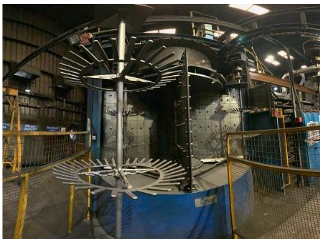
Spencer & Halstead rotary 4 compartment shot blast machine
