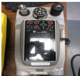
GE Druk Genii DPI620 advanced modular calibrator (2014)
