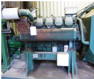
Sigmund Pulsometer fire engine pump with Fiat engine (2-off)
