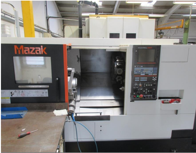
Mazak Quick Turn Smart 350M CNC slant bed turning centre (2015), Mazatrol Smart control, 12 station turret with live tooling
