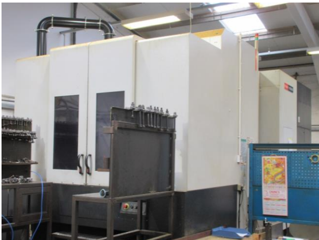
Mazak Nexus HCM - 6800 II twin pallet CNC horizontal machining centre (2008), Mazatrol Matrix Nexus control, 120 ATC
