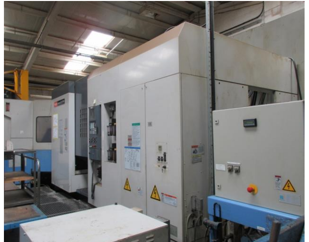
Mazak Mazatech FH-7800 5 pallet CNC horizontal machining centre (2002), Mazatrol Fusion 640m control, 180 ATC, with swarf conveyor and coolant clarifier
