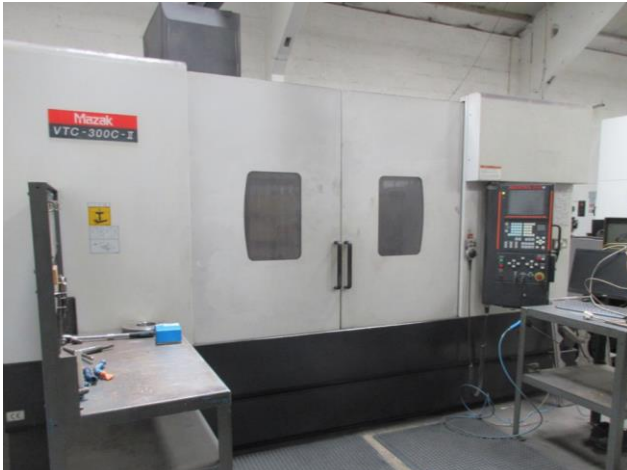
Mazak VTC-300C-II vertical machining centre, serial no. 212034 (2009), Mazatrol 640m control, 48 ATC
