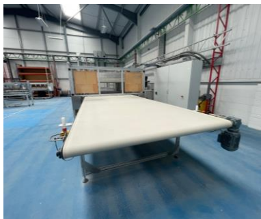
The Vac Company HVV-1300-2000 vacuum insulated panel production with belt feed conveyors (2-off 2022 & 2016, 1 x un-used)
