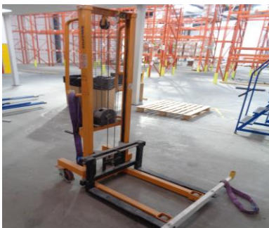
Total Lifter 250kg winch stacker (2-off)
