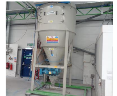
Dustcheck SFJC9, SFKJC30, SFJCO dust extraction systems (8-off, 2016 to 2021)
