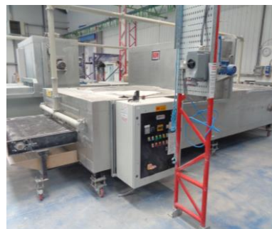
RDM SOP 69338 & SOP 63286 through feed electric tunnel ovens (4-off, 2022 to 2016, 1 x un-used)
