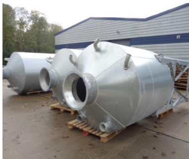
2200mm diameter steel holding silos (4-off)
