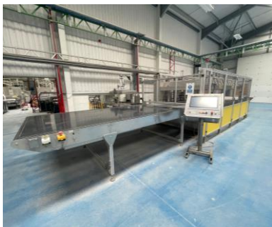
The Vac Company HVV-1300-2000 vacuum insulated panel production with belt feed conveyors (2-off 2022 & 2016, 1 x un-used)
