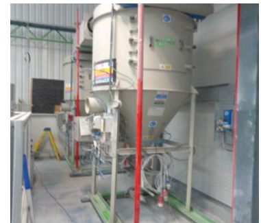
Dustcheck SFJC9, SFKJC30, SFJCO dust extraction systems (8-off, 2016 to 2021)
