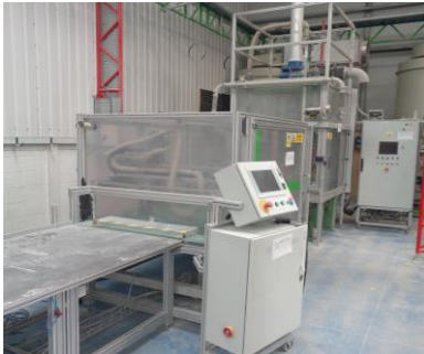
Gasbarre 28ton electronic insulation board presses with bridge type saws (4 off, 1 x un-used)
