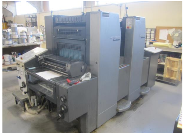
Heidelberg Speedmaster SM 52-2 2 colour offset lithographic printing press, s/n: 206432 (2003), sheet size: 370x520mm, impression count: 69.5 million
