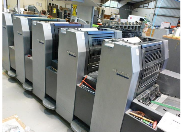
Heidelberg Speedmaster SM 52-2, 5 colour offset lithographic printing press, s/n: 207428 (2005) , with Grafix Alphatronic 200 powder spray, impression count: 81.5 million
