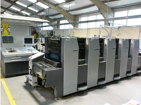
Heidelberg Speedmaster SM 52-2, 5 colour offset lithographic printing press, s/n: 207428 (2005) , with Grafix Alphatronic 200 powder spray, impression count: 81.5 million
