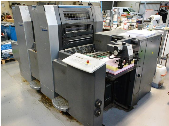
Heidelberg Speedmaster SM 52-2 2 colour offset lithographic printing press, s/n: 206432 (2003), sheet size: 370x520mm, impression count: 69.5 million
