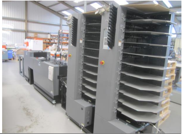
Duplo 600I Booklet maker, s/n:150700848 (installed in 2018 – Set count: 1,278,275)
