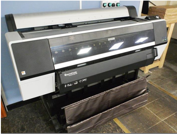
Epson Surecolour P8000 Wide format photo printer, max sheet size: A0 (2016)
