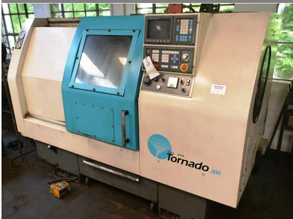
Colchester Tornado 300 slant bed CNC lathe, serial no. C30042 (1995), GE Fanuc Series 0-T control, 8 station rotary turret tailstock and 3 jaw chuck
