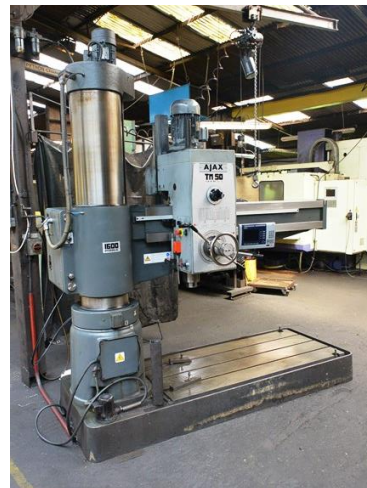
Ajax 1600mm elevating column radial arm drill, model TM50 Series 3/1600 Hydrobloc, serial no. 40008 (2007), radial digital read out
