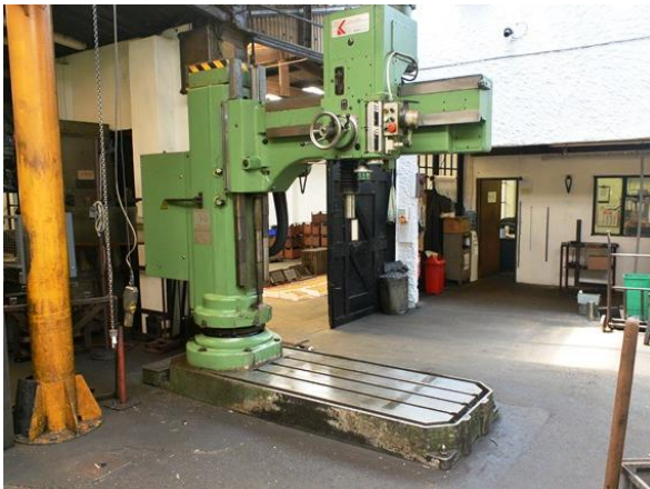
Kitchen & Walker KWM50-1600 elevating column radial arm drill, serial no. 3620 (1997), rise & fall arm.
