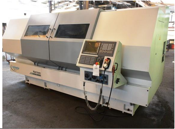
Colchester / Harrison Alpha 1660 XS CNC SS & SC gap bed centre lathe, serial no. X85015 (2020), max rpm 2000, Fanuc Series Oi-TF control, fitted rotary 8 station turret tailstock, 3 jaw chuck
