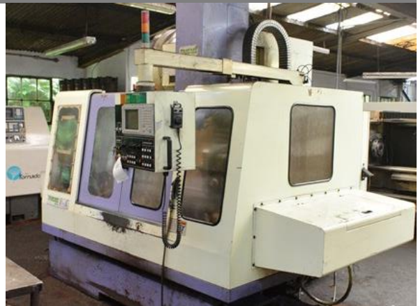
Takumi Serki V11A CNC vertical machining centre, serial no. G0698 (1998), non branded controller, table size 1350 x 500mm, 24 station ATC, fitted 4 axis
