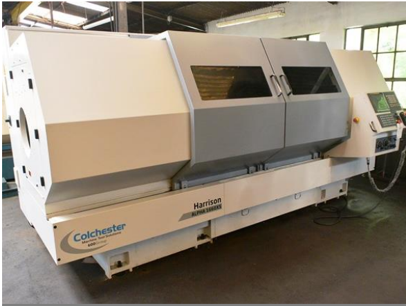
Colchester / Harrison Alpha 1660 XS CNC SS & SC gap bed centre lathe, serial no. X85015 (2020), max rpm 2000, Fanuc Series Oi-TF control, fitted rotary 8 station turret tailstock, 3 jaw chuck
