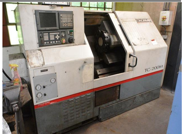
Cincinnati TC-200M CNC slant bed CNC lathe, serial no. 7052-F00-KK0157
