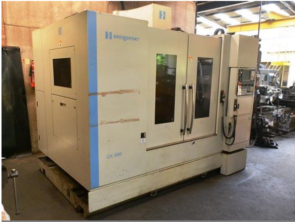
Hardinge Bridgeport GX 1000 CNC 3 axis vertical machining centre, serial no. NVCB1D0061 (2011), Fanuc Series Oi-MD, 20 ATC, table size 1120 x 540mm, max spindle speed 8000 rpm
