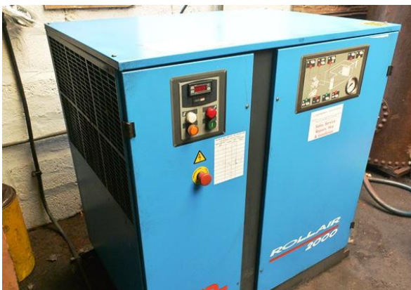
Worthington Creyssensac Rollair 2000 packaged rotary screw air compressor set, model RLR 2000 AE7, serial no. 6730372300/WCO0053112
