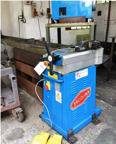
Ercolina TB-76 hydraulic tube bender, serial no. 3307044 (2007), with separate table on feed system
