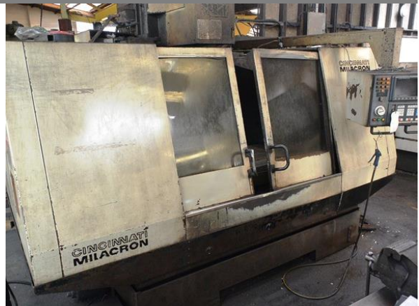
Cincinnati Milacron Sabre CNC vertical machining centre, serial no. 7037-800-RH-0162, GE Fanuc Series O-M control, ATC, table size 1350 x 650mm
