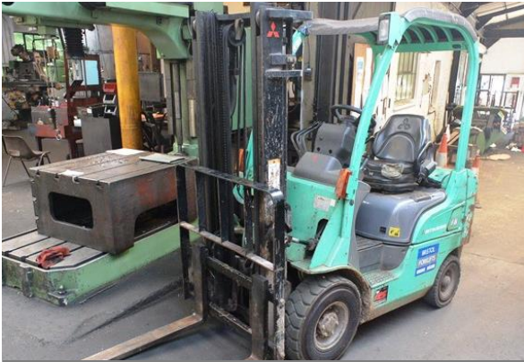
Mitsubishi 1800kg diesel ride on, dual mast forklift truck, model FD18N, serial no. EF16D 40285 (2008)
