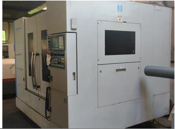
Hardinge Bridgeport GX 1000 CNC 3 axis vertical machining centre, serial no. NVCB1D0061 (2011), Fanuc Series Oi-MD, 20 ATC, table size 1120 x 540mm, max spindle speed 8000 rpm
