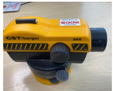
CST/Berger SAL series automatic level 24x
