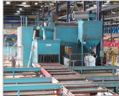
Gietart GW1500-615 blasting and top coating line
